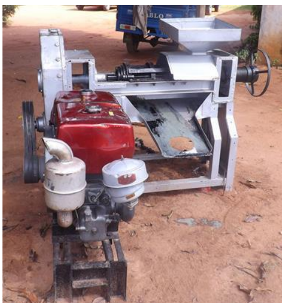
Figure 1. Presse à vis continue (Expeller)
