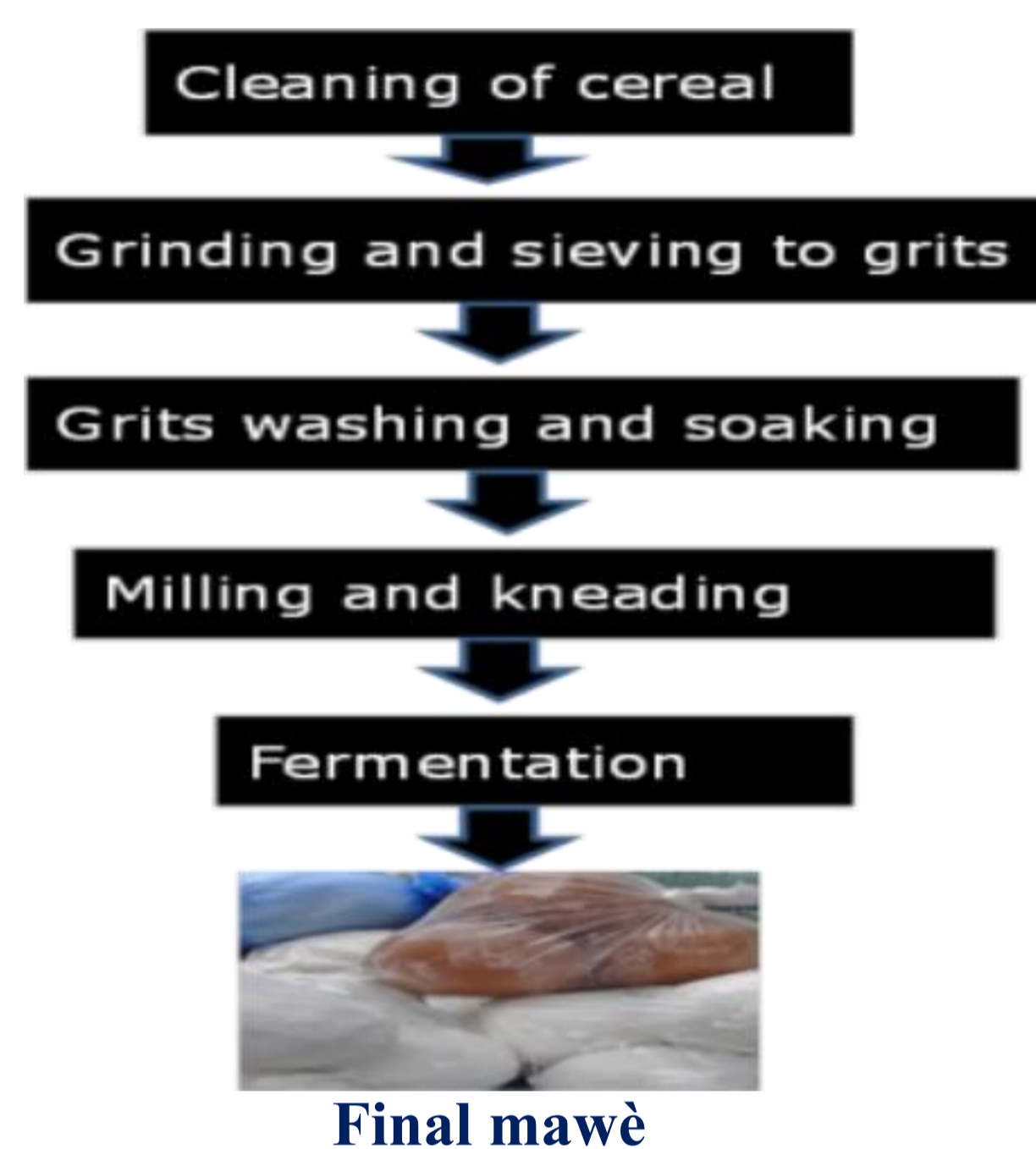
Fig. 1. Diagram flow of mawè production. The grits in not washed in home mawè processing. In come mawè processing, the cleaned maize is directly soaked in boiled water without grinding.
